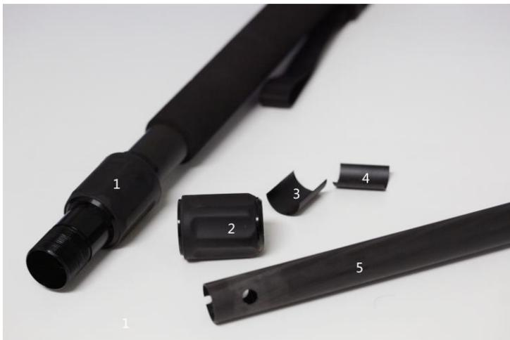
As you can see, there are 5 parts to the Sirui leg locking system. The upper leg section (#1), the locking knob (#2), a basic shim (#3), a shim with reference key (#4) and the lower leg section (#5).
