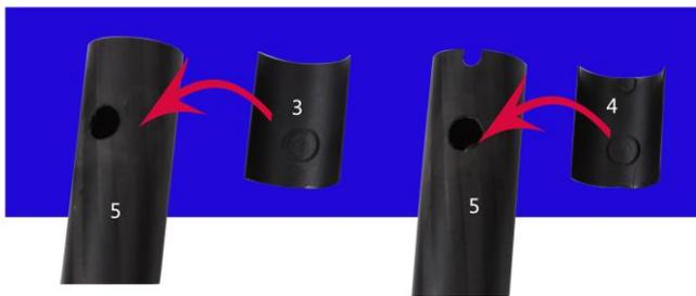
Basic shim #3 has a positioning circle that matches the hole in the lower leg section (#5). The shim (#4) has a positioning circle and reference key (a half circle on the top of the shim) that fits into the other side of the lower leg section.
